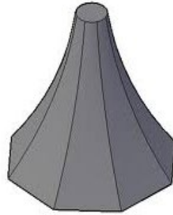
Cross sections for lofting
